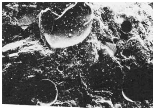
Fig. 14. Fractograph ( \times 123 ) of a mortar-PMMA composite cured at 10 days of irradiation showing a broken void (upper top) with a reasonably thick layer of PMMA firmly adhered to it, indicating a strong interfacial bonding between mortar and PMMA. The broken polymer shell bears the typical impression of a brittle fracture.
